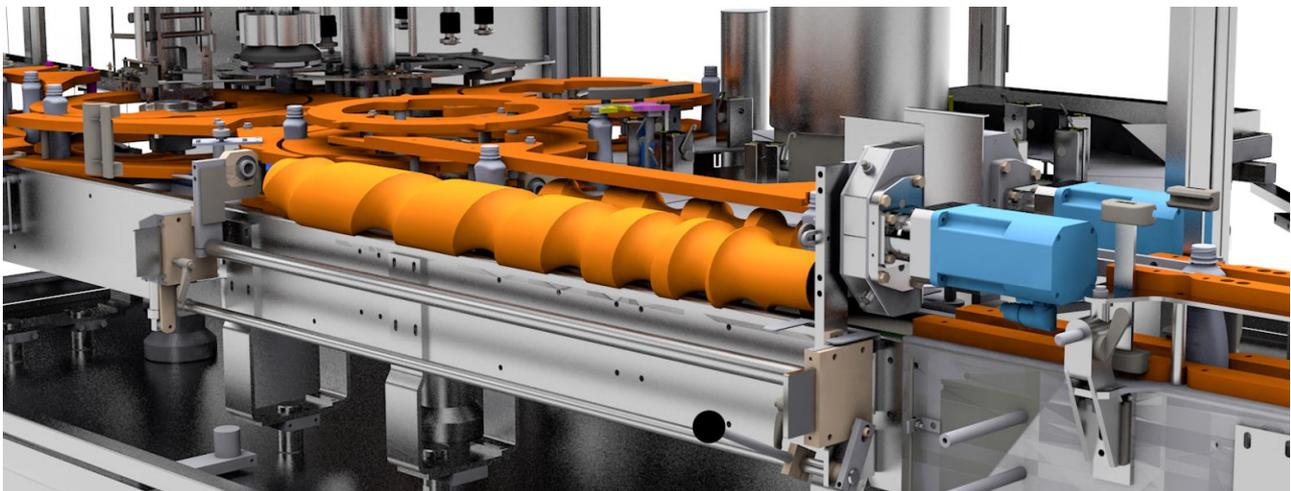
Figure 2 : Brushless containers entry timing screw
